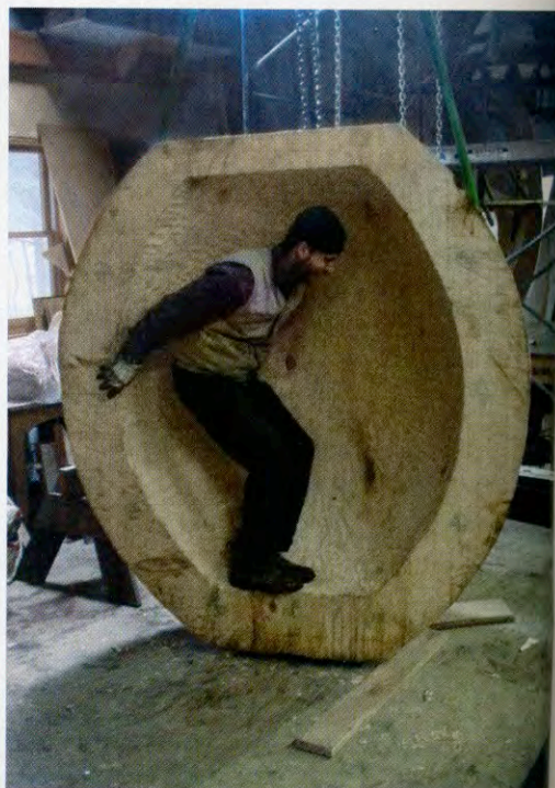
Rick Brown, far left, helps split a spruce log that was hollowed out to form Turtle 's "shells," below left. Artist Matt Hincman, below right, demonstrates the vessel's dimensions. A drawing of Turtle done in 1875, facing page, depicts a roomier sub, and illustrates the perils of historical reconstruction by including propellers of a type not invented until the 19th century, long after the British destroyed Turtle . In re-creating the sub's components, like its brass hatch, facing page, the Browns used only 18th-century techniques.
